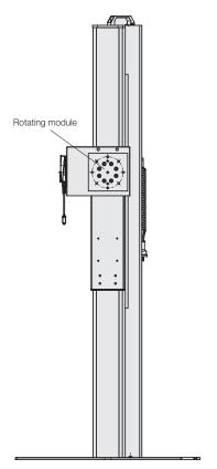
Rotating module mounted on lifting module with cart module (available on request)
