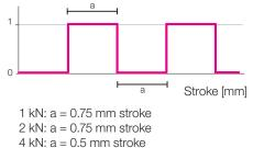
4 kN: a = 0.5 mm stroke6 kN: a = 0.375 mm stroke
