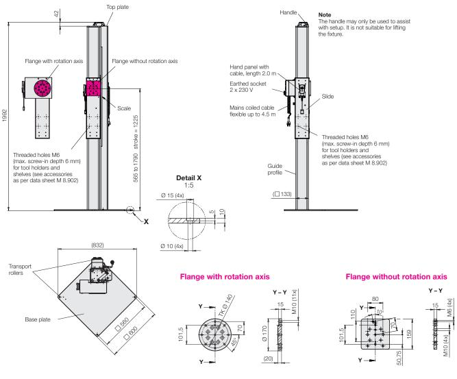
With internal threads for screwing on the universal fixture for clamping claws and 3-point pick-up.
